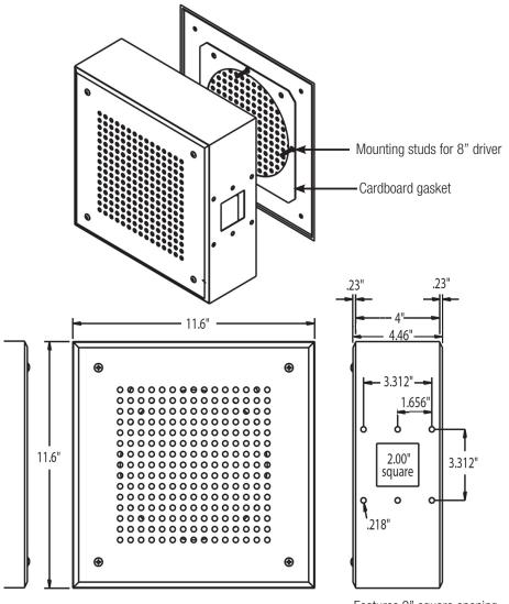
Features 2" square opening and holes for flush installation to a standard E.O. box (not included)
