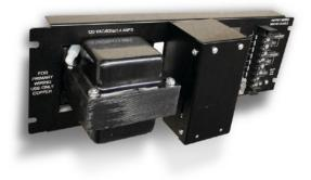
The AC Clock Power Supply provides a convenient 24Vac source for operating synchronous clocks and bells. The low voltage and current output of this power supply allows Class 2 wiring to be used. An onboard relay allows clock correction coils to be easily interfaced with Edwards master clocks. This supply mounts with the standard Edwards power supply backbox and doors.
