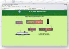
Dukane wireless clock solutions comprise a reliable master/slave mesh network that synchronizes clocks from a central on-site master controller. The master receives highly accurate time signals from an NTP or GPS source, and relays timecodes to local slave clocks via wireless signals.
