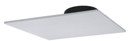
LT SERIES SPEAKERS are pro systems made for quick installation in suspended lay-in tile ceilings. The 2x2 assembly replaces a 2x2 ceiling tile. This model features an 8-inch 15W dual cone driver, 25V/70V dual voltage transformer, 2x2 white grille with black subplate and 0.147 cu.ft. enclosure.
