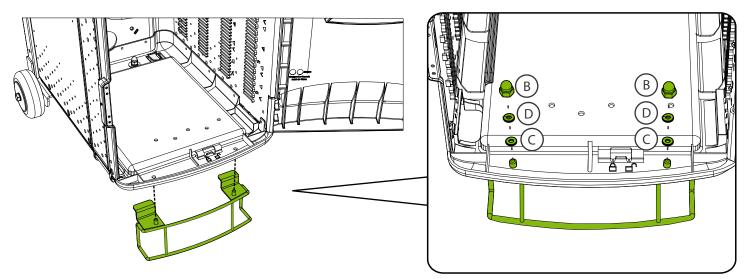
Note the orientation of the Front Support before installation.
