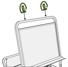
Place empty hardware bags over the top bar of the Upper Frame during instillation of Chart Paper Loop Hooks to prevent scratching. Remove bags once instillation is complete.
