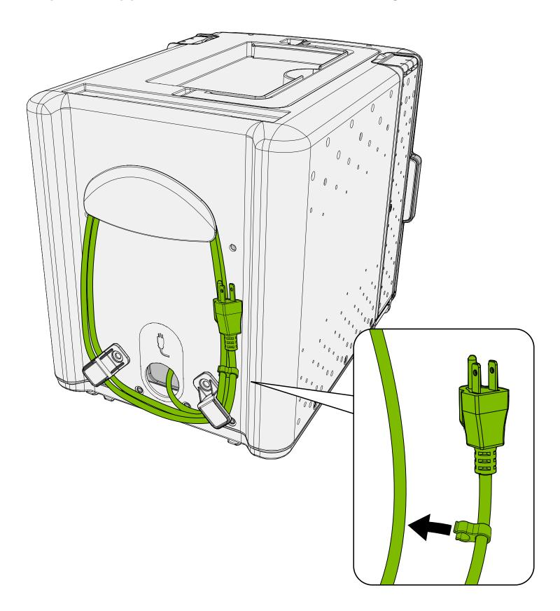
Wrap Power Strip power cable around cable hooks when moving Tech  ${\rm Tub}^{2^{\otimes}}$
