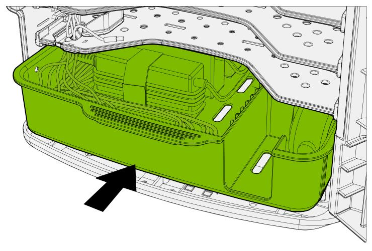
🔶 When pushing the tray in, pull the cable to keep it out of the way of the tray
