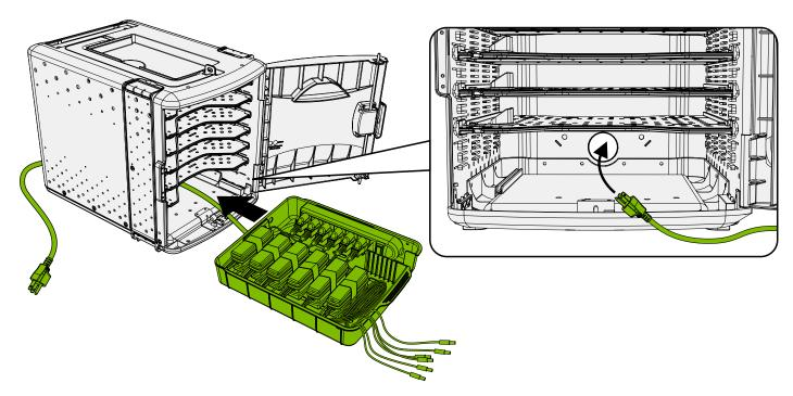
**2** Partially slide Tray back into tub (leave a gap as shown below)
