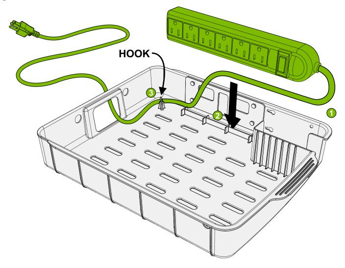
Fit 4 keyholes on Power Strip over 4 pegs on Power Strip Mounting Plate
