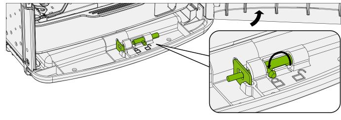
Close and lock front door of Tech Tub<sup>2'</sup> to secure devices
