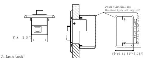
If the opening is too small or too large, the WP-700-AM cannot be mounted in the wall. Be sure to make an opening with dimensions given above when mounting.
