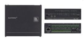
The SL-12 is a master room controller that can operate over Ethernet (LAN) with control ports that include: one bidirectional RS-485, four RS-232, four IR, four GPI/O, and eight relay. It controls devices such as scalers, video displays, audio amplifiers, DVD players, sensors, screens, shades, door locks, and lights. Multiple Kramer Ethernet gateways can be used to add remote I/O ports.
