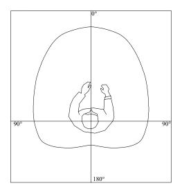
FIG. 4 - This polar plot shows the relative level from a talker versus angle. The speech level at a listener's position decreases by approximately 1.5dB for every 30° the talker is off-axis from the listener. The orientation of the listener's head is unimportant in speech level calculations.
