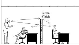
FIG. 5 - Screens should (a) be high enough to reduce sound passing over them, (b) provide a good barrier to sounds passing through them, and (c) absorb incident sound.
