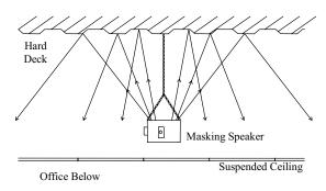
FIG. 13 - Typical masking loudspeaker suspended in a ceiling plenum with a hard deck.
