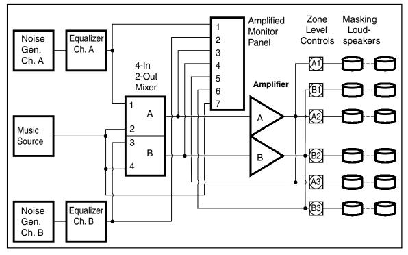
FIG. 12 - Wiring diagram of a two-channel sound-masking system with zone level controls, background music, and an amplified monitor panel.
