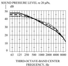
FIG. 20 - Comparison of Masking Spectra: Sound Masking Spectrum 1 \_\_\_\_\_ (preferred)
