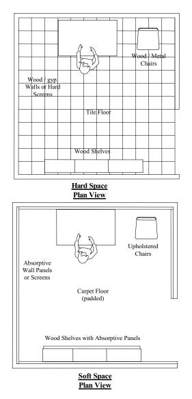
FIG. 9 - Use absorptive office furnishings and thick, padded carpet to reduce unwanted reflected sound.
