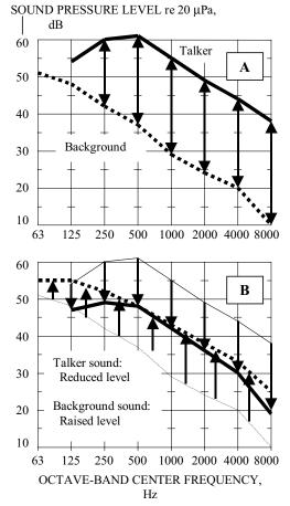
FIG. 2 - This two-part graph illustrates the concept of sound masking by showing octave-band sound levels of a talker and background sound before (Part A) and after (Part B) acoustical improvements and sound masking are installed.
