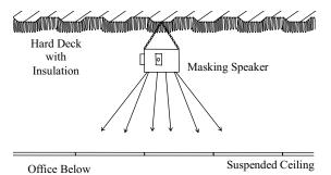
FIG. 14 - If the underside of the deck is absorptive because of sprayed-on thermal insulation (top floor of many buildings), mount the masking loudspeakers as high as possible and point them downwards. This configuration requires more loudspeakers to maintain even coverage.
