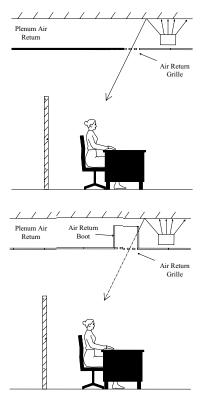
FIG. 8 - Install boots above open return air ducts in ceiling plenums.
