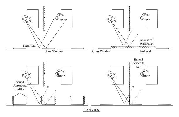
FIG. 10 - Walls, doors, windows and curtain walls can reflect sound into adjacent workstations.
