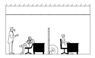
FIG. 15 - A self-contained masking unit used as a "spot" masker in an office.
