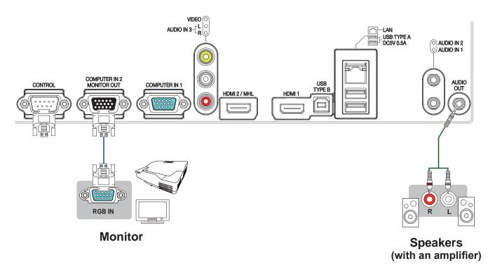
To use network functions of the projector, connect the **LAN** port with the computer's LAN port, or with an access point that is connected to the computer with wireless LAN, using a LAN cable. To use NETWORK BRIDGE function, also connect the **CONTROL** port and an RS-232C port of the external device to communicate as a network terminal. See the **User's Manual - Network Guide** for details of the network functions.
