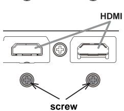
It is recommended to fasten the HDMI cables by using the HDMI cable holder and the Cable tie to prevent them from coming off. Use a Cable tie with the size of 2.0 x 4.0mm or smaller.
