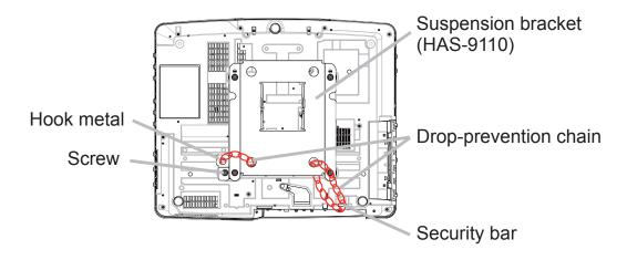
Pass the drop-prevention chain through the hole of the optional suspension bracket and hook metal, and fix it securely with a quick link.
